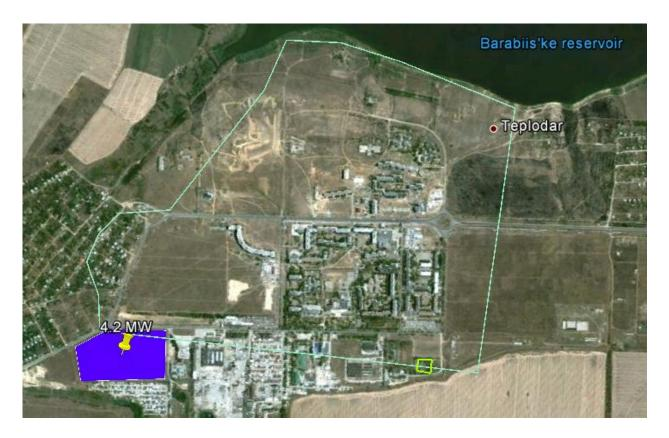
The project will install 17,182 solar PV modules each having 245 Wp capacity, as well as 12 inverters each having a nominal capacity of 330 KWp. The planned installed capacity of the project will be 4.209 megawatt, which will provide an annual gross electricity generation of 4,916 MW-hours.
