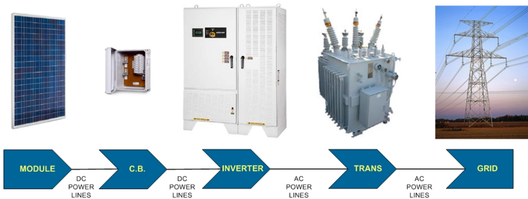
Figure 3-2. Typical PV Components
